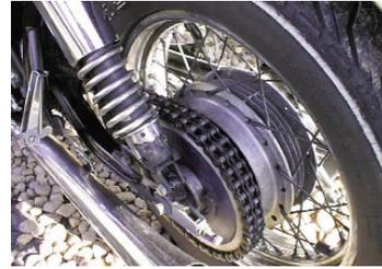
A rider will recognize a chain break due to the instant loss of power to the cycle's rear wheel. If this situation should arise, roll off and close the throttle while gently braking to a safe stop at the road's edge. Chain slippage or breakage can be avoided through routine and proper maintenance.
